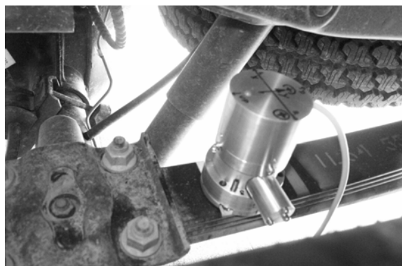
Figure 3 – Optical Rousette measuring the stress/strain in a truck suspension and a software result
